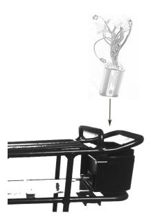
Connect the RED and BLACK battery wires on the controller to the corresponding colours in the controller box. For a full controller connections guide, please refer to your eKit User Manual.
