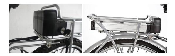
The battery should slide in and out easily through the rail at the bottom of the pannier rack. In case the battery doesn't slide all the way in and, as a result, you are having difficulties locking the battery in place with the ignition key, this is likely because you have not aligned the controller box on the pannier rack properly. Please perform the following steps to align the controller box:
